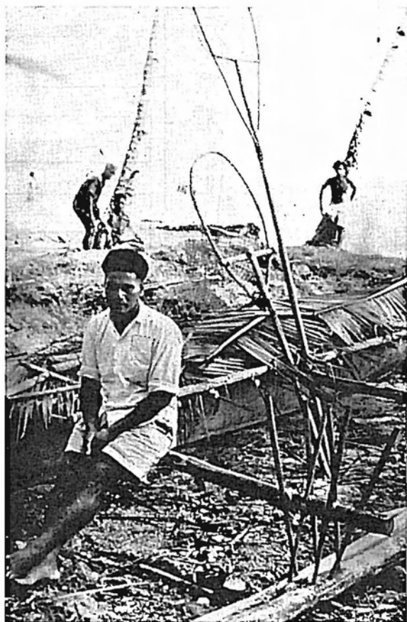
Fig 55. Baka 'eha canoe on its landing place. The hull is protected against sun by a coconut leaf cover. Notice the strong, yet flexible fastening of the outrigger float to the booms by means of sticks. A short- and a long-handled kupenga -net is also seen.
